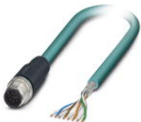
Assembled Ethernet cable, shielded, 4-pair, 26 AWG stranded (7-wire), RAL 5021 (water blue), M12 male plug to free cable end, line, length: 4 m
