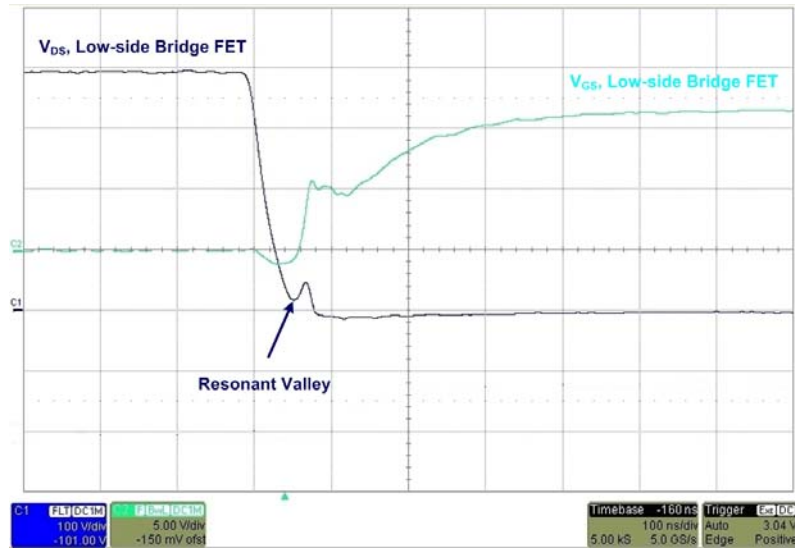
FIGURE 21. RESONANT SWITCHING WITH 100% (50A) LOAD
