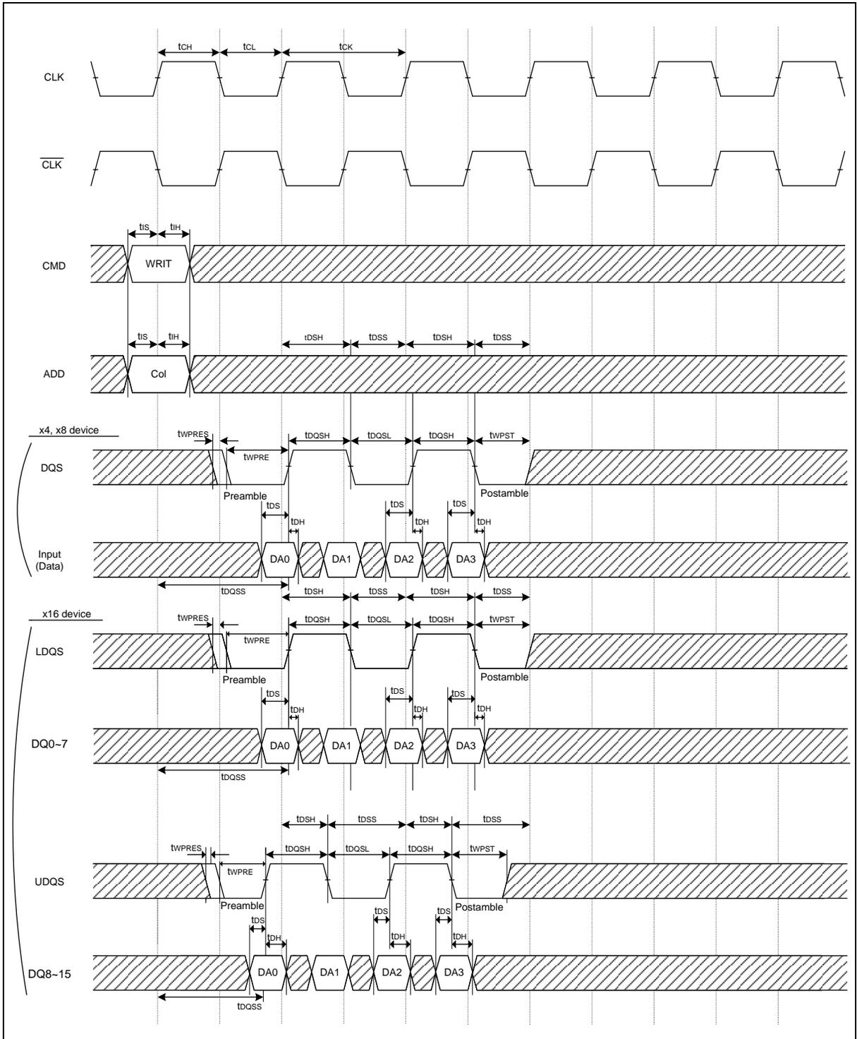
**Note:** x16 has two DQs (UDQS for upper byte and LDQS for lower byte). Even if one of the 2 bytes is not used, both UDQS and LDQS must be toggled.
