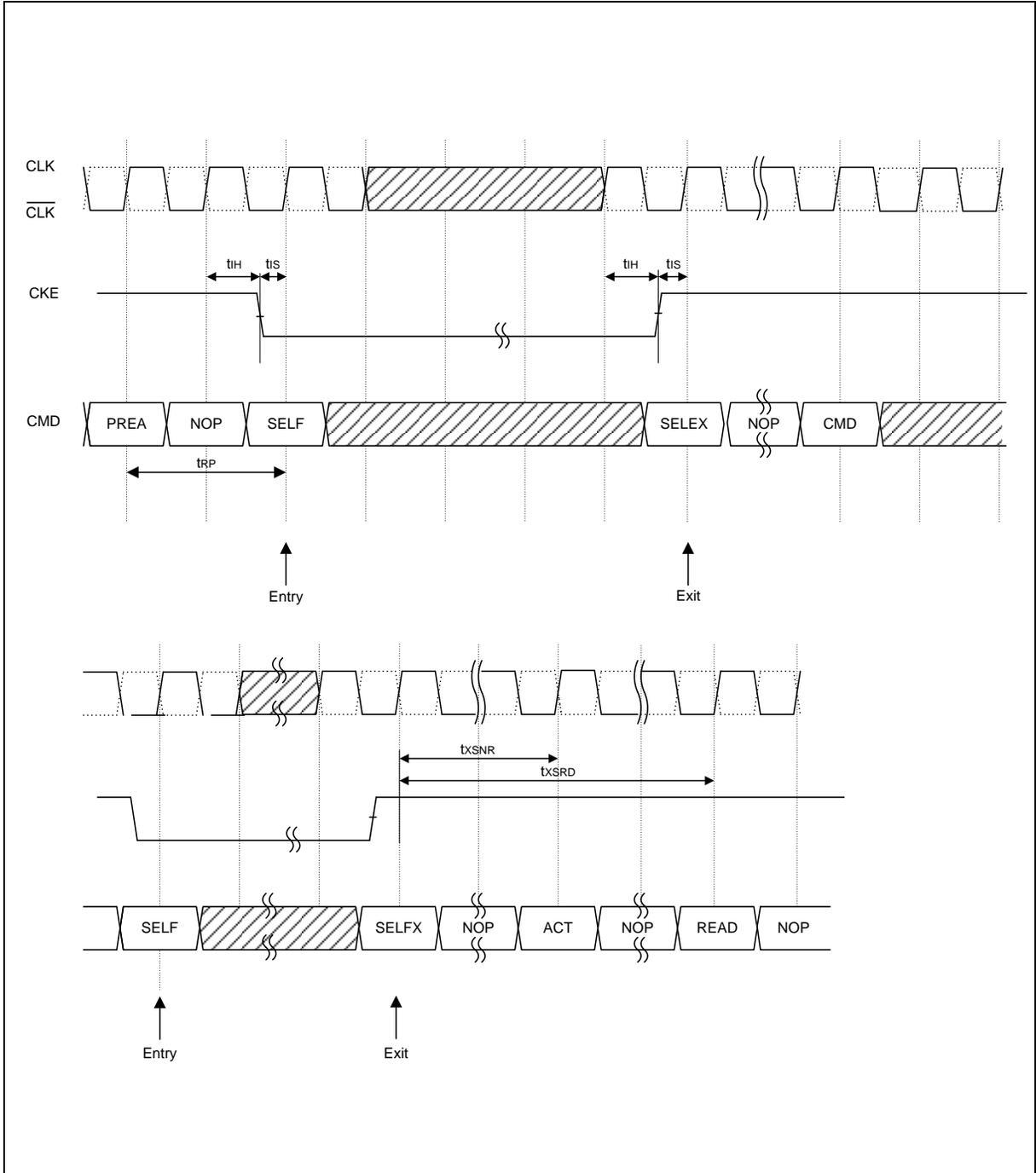
**Note:** If the clock frequency is changed during self refresh mode, a DLL reset is required upon exit.
