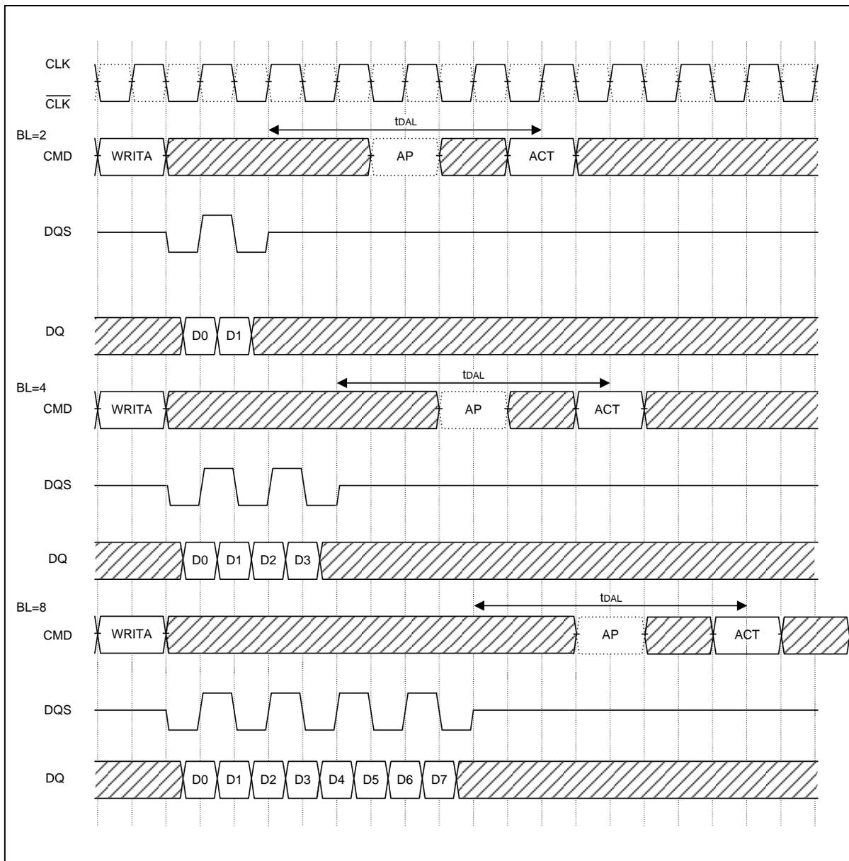
The Write with Auto-precharge command cannot be interrupted by any other command.
