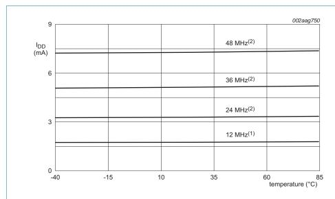
Conditions:  $V_{DD} = 3.3 \text{ V}$ ; Active mode entered executing code while(1) {} from flash; internal pull-up resistors disabled; BOD disabled; all peripherals disabled in the SYSAHBCLKCTRL register; all peripheral clocks disabled; low-current mode; USB\_DP and USB\_DM pulled LOW externally.
