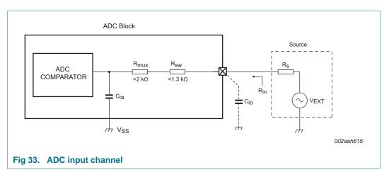
The effective input impedance,  $R_{in}$ , seen by the external voltage source,  $V_{EXT}$ , is the parallel impedance of ((1/f<sub>s</sub> x C<sub>ia</sub>) +  $R_{mux}$  +  $R_{sw}$ ) and (1/f<sub>s</sub> x C<sub>io</sub>), and can be calculated using Equation 1 with
