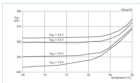
Conditions: BOD disabled; all oscillators and analog blocks turned off in the PDSLEEPCFG register; USB\_DP and USB\_DM pulled LOW externally.
