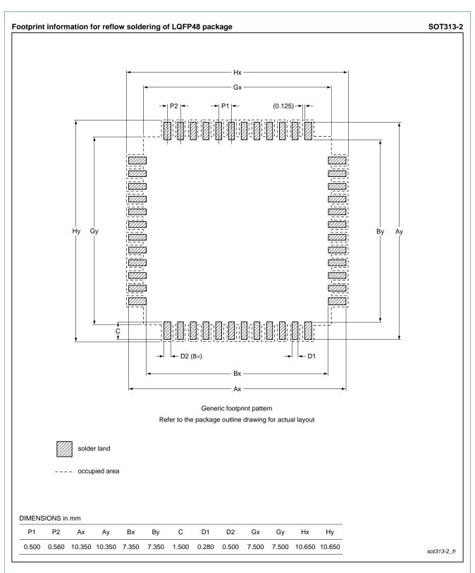
Fig 42. Reflow soldering for the LQFP48 package
