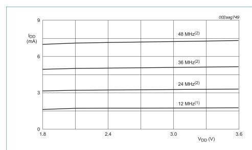
Conditions:  $T_{amb} = 25$  °C; Active mode entered executing code while (1) {} from flash; internal pull-up resistors disabled; BOD disabled; all peripherals disabled in the SYSAHBCLKCTRL register; all peripheral clocks disabled; low-current mode; USB\_DP and USB\_DM pulled LOW externally.
