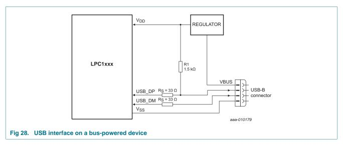
**Remark:** When a bus-powered circuit as shown in Figure 28 is used, configure the PIO0\_3/USB\_VBUS pin for GPIO (PIO0\_3) in the IOCON block to ensure that the USB\_CONNECT signal can still be controlled by software. For details on the soft-connect feature, see the *LPC11U3x user manual* (Ref. 1).
