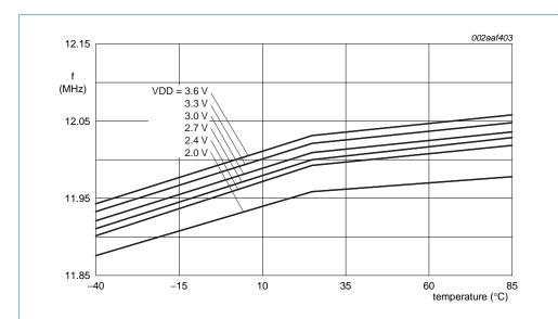
Conditions: Frequency values are typical values. 12 MHz  $\pm$  1 % accuracy is guaranteed for 2.7 V  $\leq$  V<sub>DD</sub>  $\leq$  3.6 V and T<sub>amb</sub> = -40 °C to +85 °C. Variations between parts may cause the IRC to fall outside the 12 MHz  $\pm$  1 % accuracy specification for voltages below 2.7 V.
