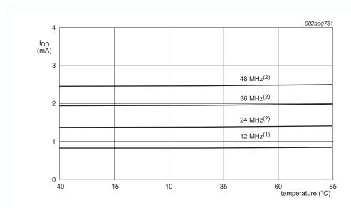
Conditions: V<sub>DD</sub> = 3.3 V; Sleep mode entered from flash; internal pull-up resistors disabled; BOD disabled; all peripherals disabled in the SYSAHBCLKCTRL register; all peripheral clocks disabled; low-current mode; USB\_DP and USB\_DM pulled LOW externally.
