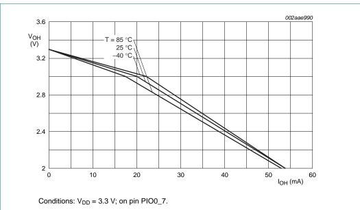
Fig 15. High-drive output: Typical HIGH-level output voltage  $V_{OH}$  versus HIGH-level output current  $I_{OH}$ .
