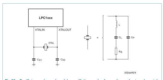
Fig 30. Oscillator modes and models: oscillation mode of operation and external crystal model used for  $C_{X1}/C_{X2}$  evaluation
