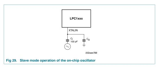
In slave mode, couple the input clock signal with a capacitor of 100 pF (<u>Figure 29</u>), with an amplitude between 200 mV (RMS) and 1000 mV (RMS). This signal corresponds to a square wave signal with a signal swing of between 280 mV and 1.4 V. The XTALOUT pin in this configuration can be left unconnected.
