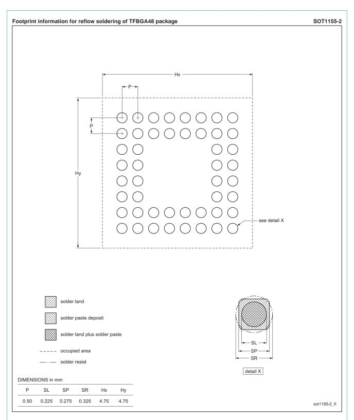
Fig 41. Reflow soldering for the TFBGA48 package
