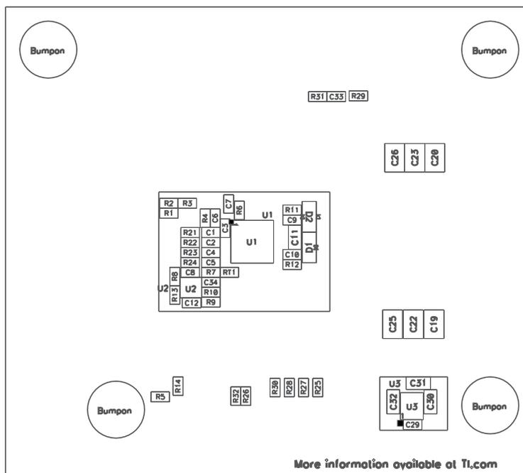
Figure 16. TPS51727EVM Bottom Assembly Drawing, Bottom View
