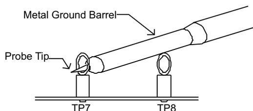
**Figure 3. Tip and Barrel Measurement for Vout Ripple**
