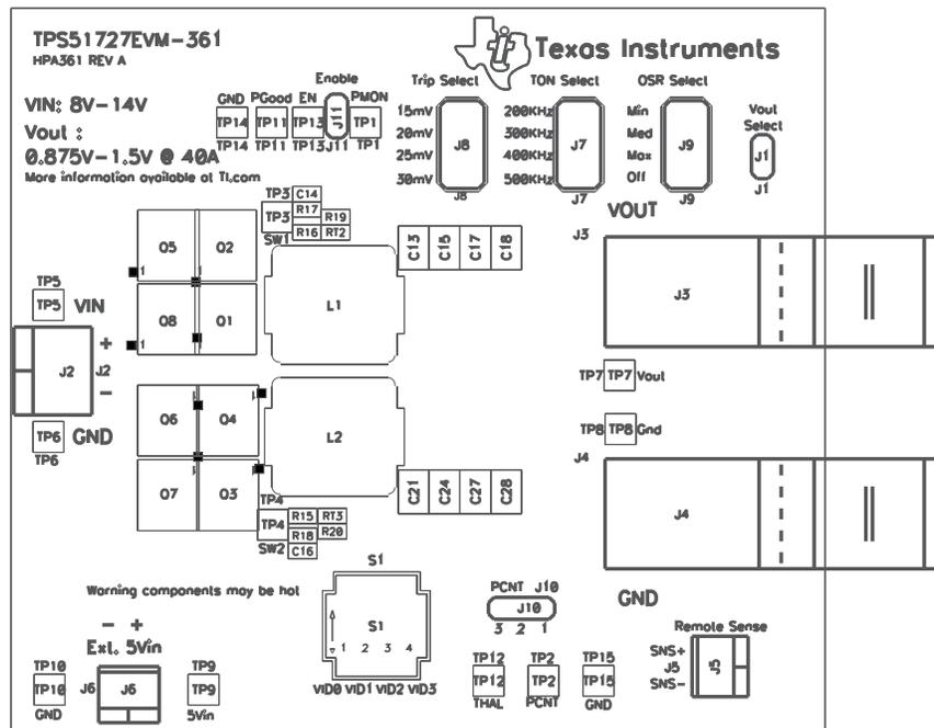
Figure 15. TPS51727EVM Top Layer Assembly Drawing, Top View
