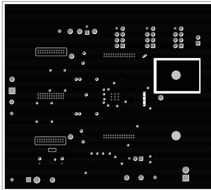
Figure 21. TPS51727EVM Internal Layer 5, Top View
