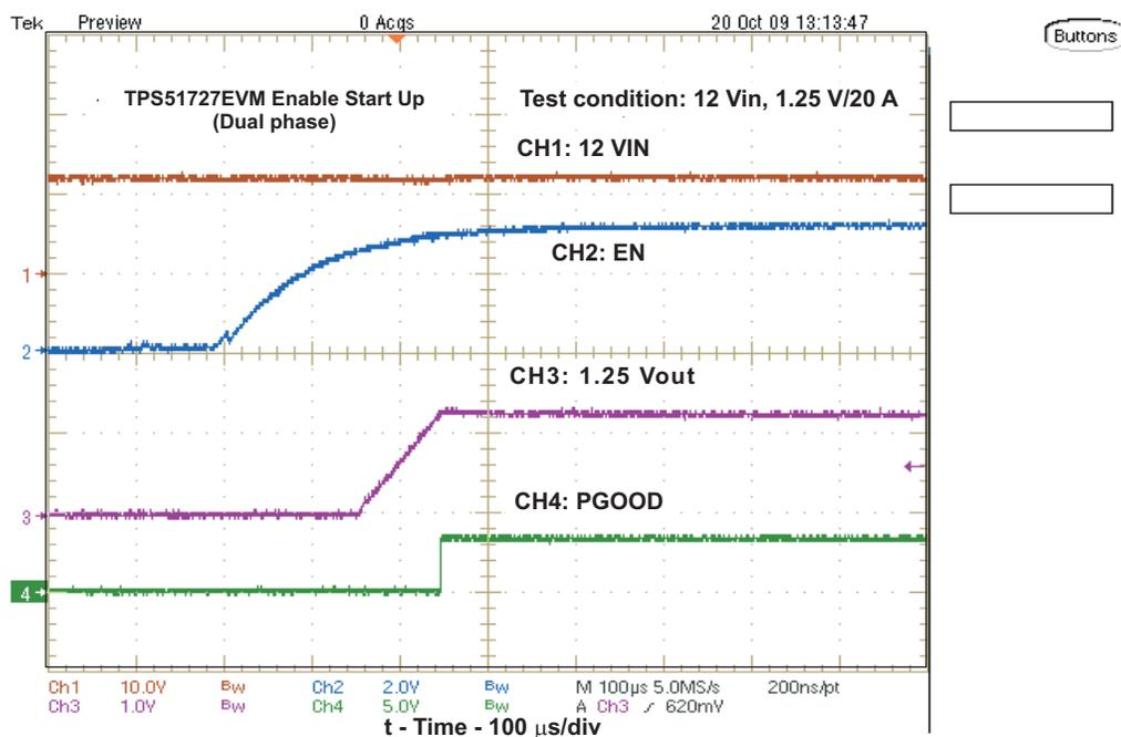
Figure 13. Enable Turnon Waveform
