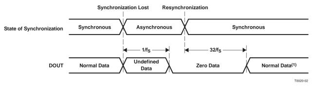
(1) The transient response (exponentially attenuated signal from ±0.2% dc of FSR with 200-ms time constant) appears initially.
