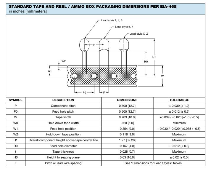
Tape and Reel Packaging: type 199D radial-leaded tantalum capacitors, all lead styles except 1, 3, and Y are available taped and reeled per EIA-468.
