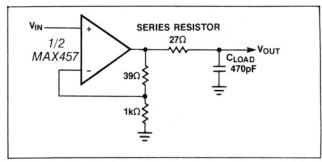
Figure 2. Isolating a Capacitive Load
