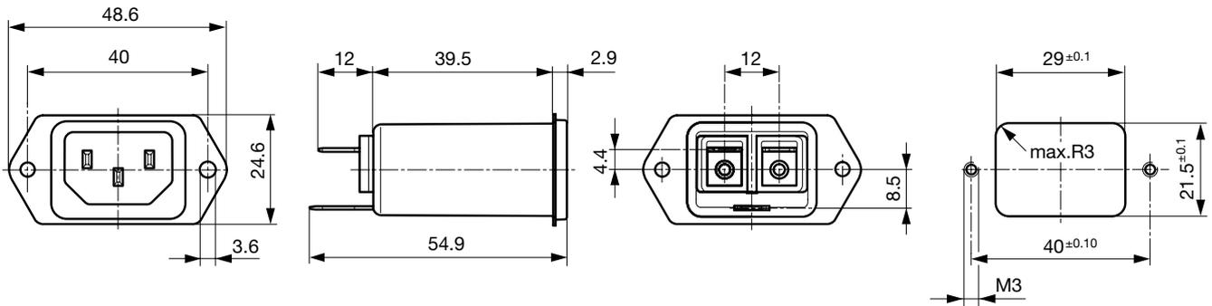
Front side mounting with plastic flange
