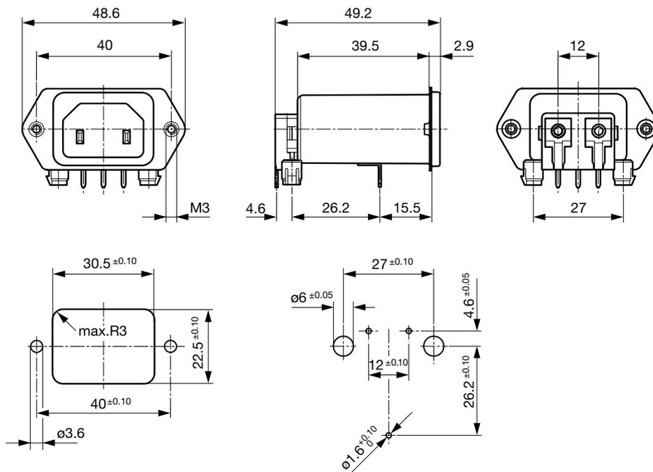
PCB rear side mounting, protection class II
