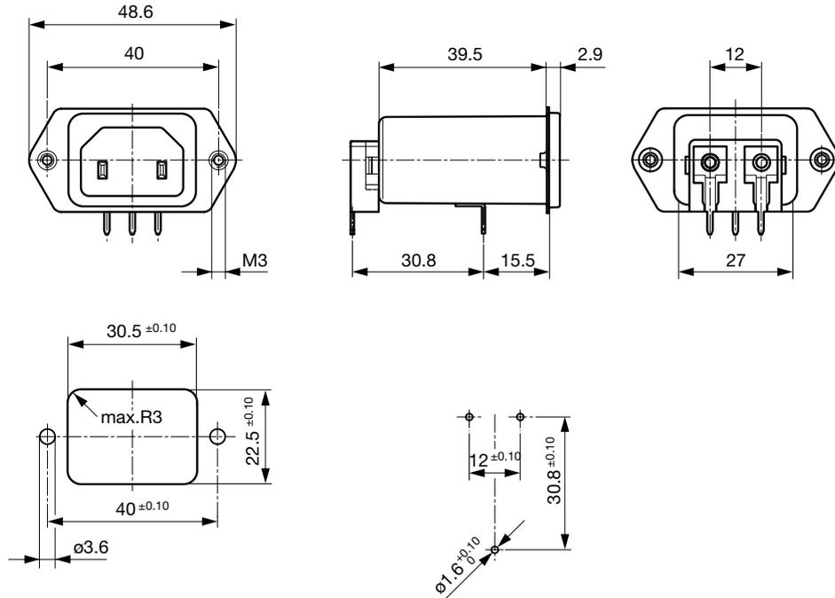
Screw and snap-in mounting with flexible wire
