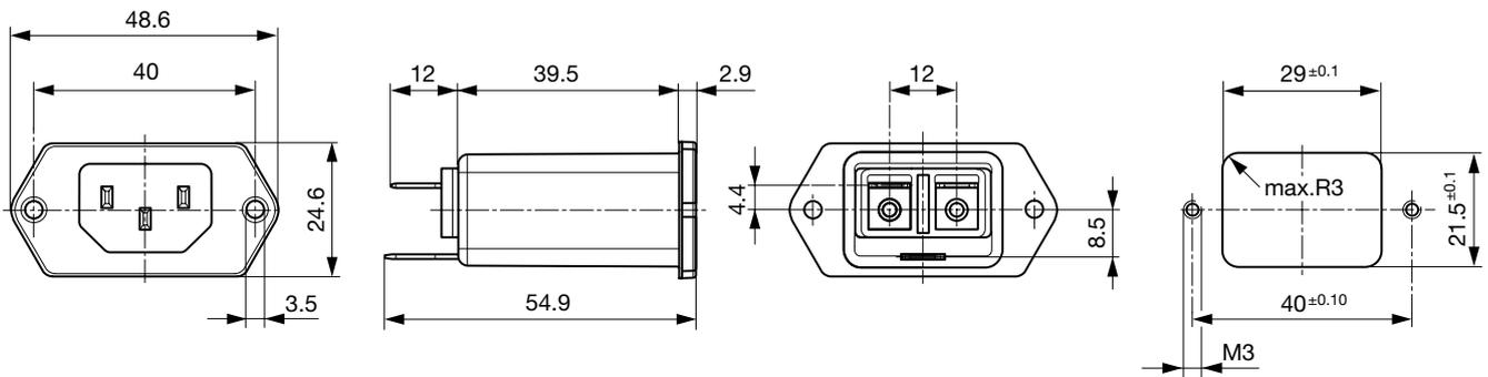
Rear side mounting with pre-formed, threaded holes for M3 screws (panel cutout for rear side mounting)
