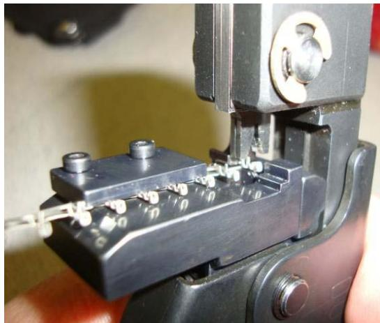
3. The terminal is located in the proper crimping area of the tooling when the “ball-detent” feature of the tool locates the feed hole of the terminal carrier strip and restricts the side-to-side movement of the strip.
