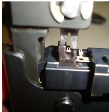
(2) Straighten wire before placing in hand-tool. Insert the stripped end of the wire into wire barrel of terminal, verifying that all conductor strands are contained within the terminal's conductor tines.
