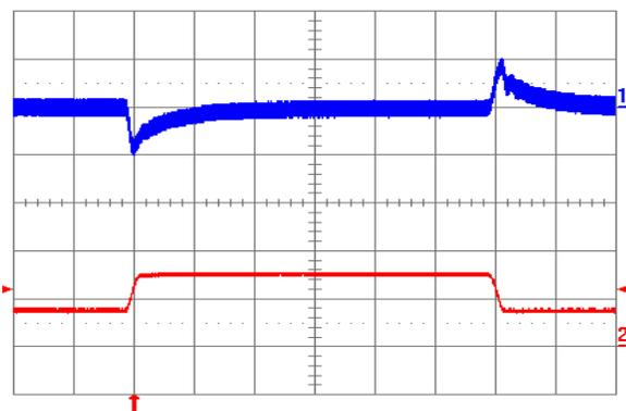
Fig. 1.5V.11: Output voltage response to load current step-change (3.75 A – 7.5 A – 3.75 A) at V<sub>in</sub> = 24V. Top trace: output voltage (100 mV/div.). Bottom trace: load current (5 A/div.). Current slew rate: 0.1 A/µs. C<sub>o</sub> = 1 µF ceramic. Time scale: 0.2 ms/div.
