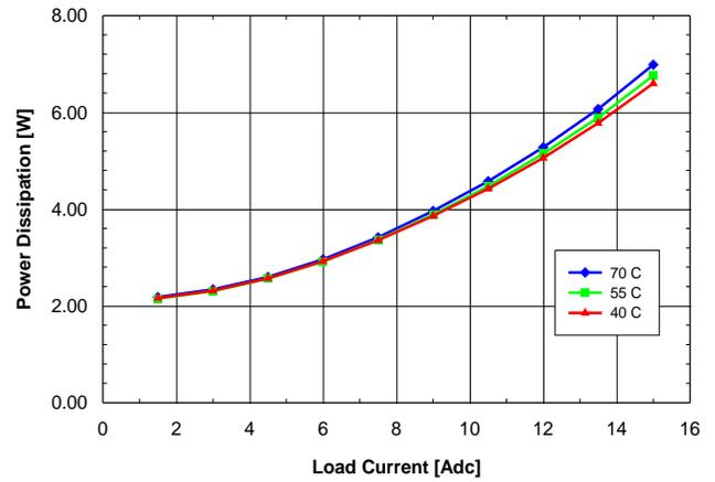
Fig. 3.3V.8: Power dissipation vs. load current and ambient temperature for SQ24T/S15033 converter mounted vertically with V<sub>in</sub> = 24V and air flowing from pin 3 to pin 1 at a rate of 200 LFM (1.0 m/s).
