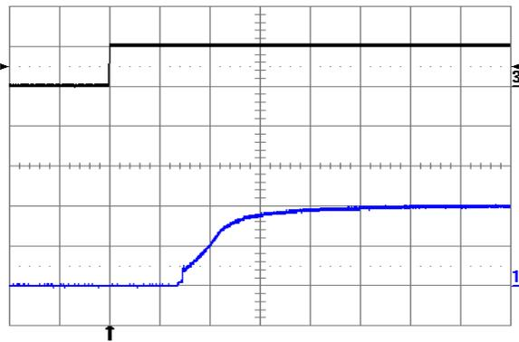
Fig. 2.0V.9: Turn-on transient at full rated load current (resistive) with no output capacitor at V<sub>in</sub> = 24V, triggered via ON/OFF pin. Top trace: ON/OFF signal (5 V/div.). Bottom trace: output voltage (1 V/div.). Time scale: 1 ms/div.
