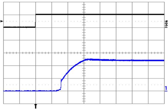
Fig. 1.2V.10: Turn-on transient at full rated load current (resistive) plus 10,000 µF at V<sub>in</sub> = 24V, triggered via ON/OFF pin. Top trace: ON/OFF signal (5 V/div.). Bottom trace: output voltage (0.5 V/div.). Time scale: 1 ms/div.
