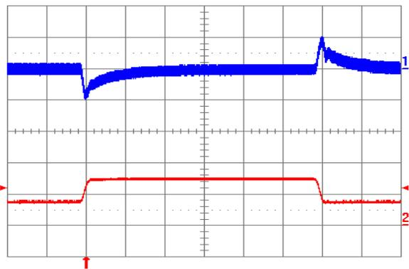
Fig. 1.2V.11: Output voltage response to load current step-change (3.75 A – 7.5 A – 3.75 A) at V<sub>in</sub> = 24V. Top trace: output voltage (100 mV/div.). Bottom trace: load current (5 A/div.). Current slew rate: 0.1 A/µs. C<sub>o</sub> = 1 µF ceramic. Time scale: 0.2 ms/div.
