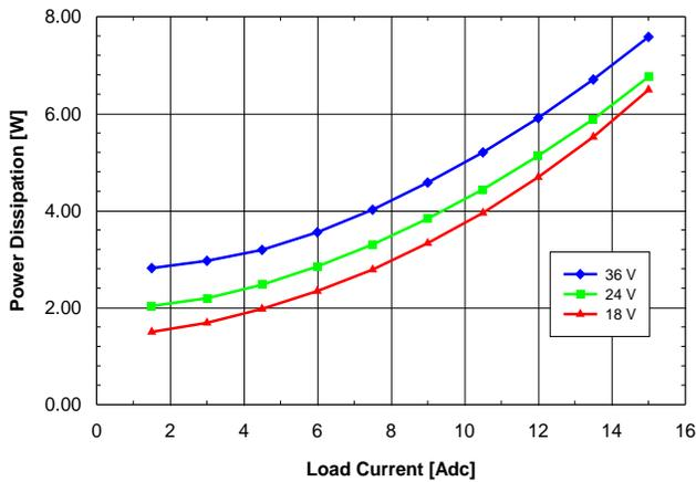
Fig. 3.3V.7: Power dissipation vs. load current and input voltage for SQ24T/S15033 converter mounted vertically with air flowing from pin 3 to pin 1 at a rate of 300 LFM (1.5 m/s) and T<sub>a</sub> = 25°C.
