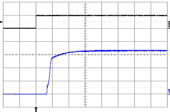
Fig. 3.3V.9: Turn-on transient at full rated load current (resistive) with no output capacitor at V<sub>in</sub> = 24V, triggered via ON/OFF pin. Top trace: ON/OFF signal (5 V/div.). Bottom trace: output voltage (1 V/div.). Time scale: 2 ms/div.
