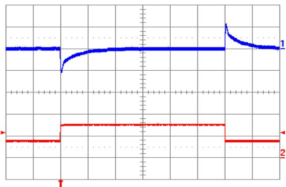
Fig. 2.5V.12: Output voltage response to load current step-change (3.75 A – 7.5 A – 3.75 A) at  $V_{in} = 24\text{V}$ . Top trace: output voltage (100 mV/div.). Bottom trace: load current (5 A/div.). Current slew rate: 5 A/ $\mu\text{s}$ .  $C_o = 450 \mu\text{F}$  tantalum + 1  $\mu\text{F}$  ceramic. Time scale: 0.2 ms/div.
