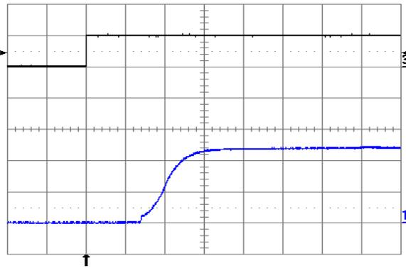
Fig. 12V.9: Turn-on transient at full rated load current (resistive) with no output capacitor at  $V_{in} = 24\text{V}$ , triggered via ON/OFF pin. Top trace: ON/OFF signal (5 V/div.). Bottom trace: output voltage (5 V/div.). Time scale: 1 ms/div.
