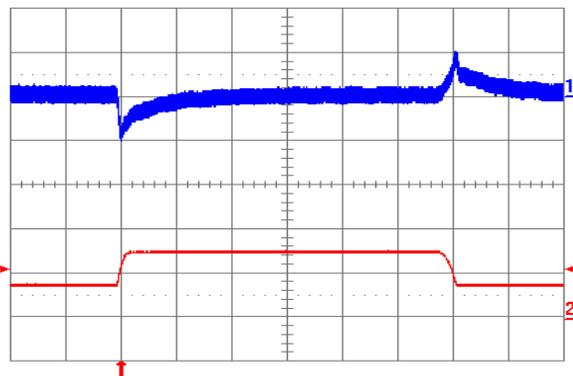
Fig. 3.3V.11: Output voltage response to load current step-change (3.75A – 7.5A – 3.75A) at V<sub>in</sub> = 24V. Top trace: output voltage (100 mV/div.). Bottom trace: load current (5 A/div.). Current slew rate: 0.1 A/µs. C<sub>o</sub> = 1 µF ceramic. Time scale: 0.2 ms/div.
