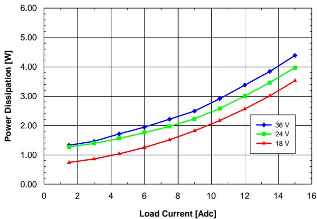
Fig. 1.0V.7: Power dissipation vs. load current and input voltage for SQ24T/S15010 converter mounted vertically with air flowing from pin 3 to pin 1 at a rate of 300 LFM (1.5 m/s) and T<sub>a</sub> = 25°C.
