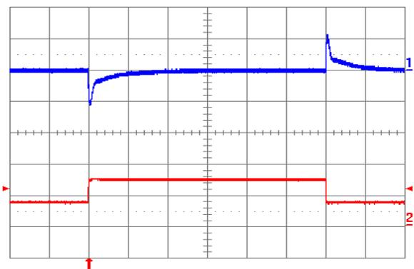
Fig. 1.0V.12: Output voltage response to load current step-change (3.75 A – 7.5 A – 3.75 A) at V<sub>in</sub> = 24V. Top trace: output voltage (100 mV/div.). Bottom trace: load current (5 A/div.). Current slew rate: 5 A/µs. C<sub>o</sub> = 450 µF tantalum + 1 µF ceramic. Time scale: 0.2 ms/div.
