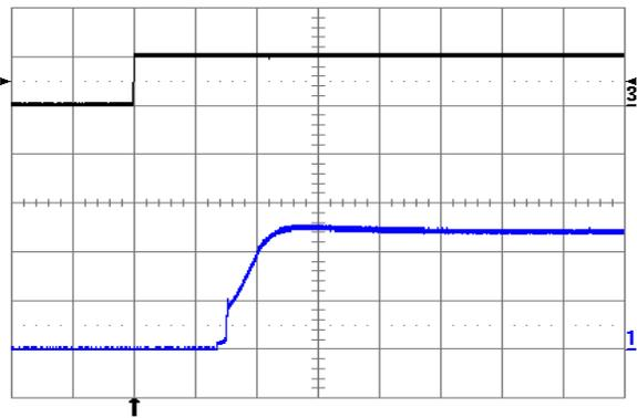
Fig. 1.2V.9: Turn-on transient at full rated load current (resistive) with no output capacitor at V<sub>in</sub> = 24V, triggered via ON/OFF pin. Top trace: ON/OFF signal (5 V/div.). Bottom trace: output voltage (0.5 V/div.). Time scale: 1 ms/div.
