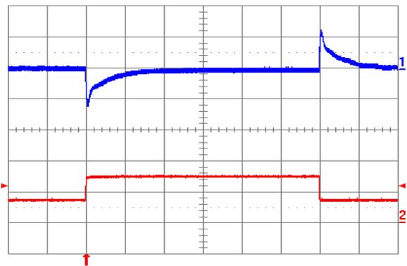
Fig. 2.0V.12: Output voltage response to load current step-change (3.75A – 7.5A – 3.75A) at V<sub>in</sub> = 24V. Top trace: output voltage (100 mV/div.). Bottom trace: load current (5 A/div.). Current slew rate: 5 A/µs. C<sub>o</sub> = 450 µF tantalum + 1 µF ceramic. Time scale: 0.2 ms/div.
