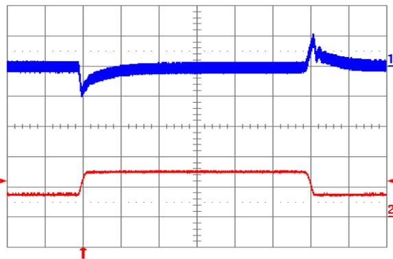
Fig. 2.0V.11: Output voltage response to load current step-change (3.75A – 7.5A – 3.75A) at V<sub>in</sub> = 24V. Top trace: output voltage (100 mV/div.). Bottom trace: load current (5 A/div.). Current slew rate: 0.1 A/µs. C<sub>o</sub> = 1 µF ceramic. Time scale: 0.2 ms/div.
