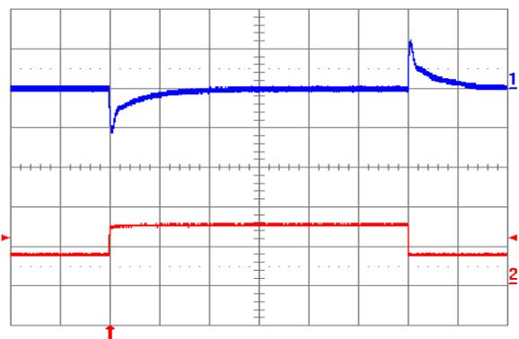
Fig. 1.5V.12: Output voltage response to load current step-change (3.75 A – 7.5 A – 3.75 A) at V<sub>in</sub> = 24V. Top trace: output voltage (100 mV/div.). Bottom trace: load current (5 A/div.). Current slew rate: 5 A/µs. C<sub>o</sub> = 450 µF tantalum + 1 µF ceramic. Time scale: 0.2 ms/div.
