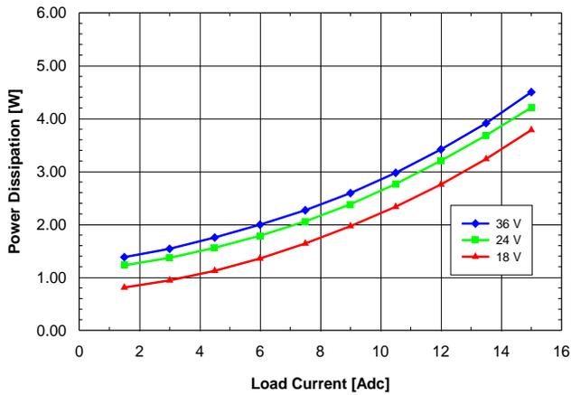
Fig. 1.2V.7: Power dissipation vs. load current and input voltage for SQ24T/S15012 converter mounted vertically with air flowing from pin 3 to pin 1 at a rate of 300 LFM (1.5 m/s) and T<sub>a</sub> = 25°C.
