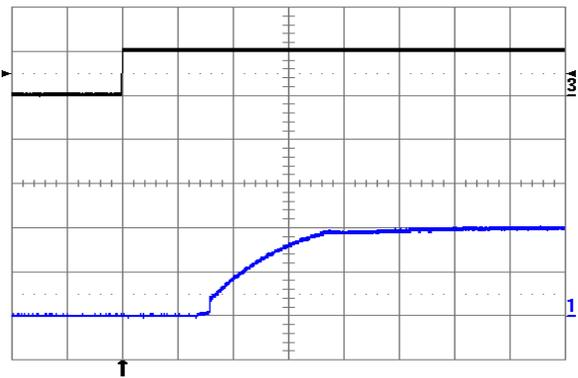
Fig. 2.0V.10: Turn-on transient at full rated load current (resistive) plus 10,000µF at V<sub>in</sub> = 24V, triggered via ON/OFF pin. Top trace: ON/OFF signal (5 V/div.). Bottom trace: output voltage (1 V/div.). Time scale: 1 ms/div.
