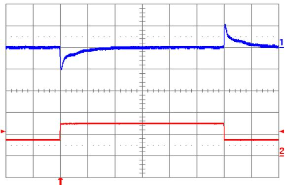
Fig. 3.3V.12: Output voltage response to load current step-change (3.75A – 7.5A – 3.75A) at V<sub>in</sub> = 24V. Top trace: output voltage (100 mV/div.). Bottom trace: load current (5 A/div.). Current slew rate: 5 A/µs. C<sub>o</sub> = 450 µF tantalum + 1 µF ceramic. Time scale: 0.2 ms/div.
