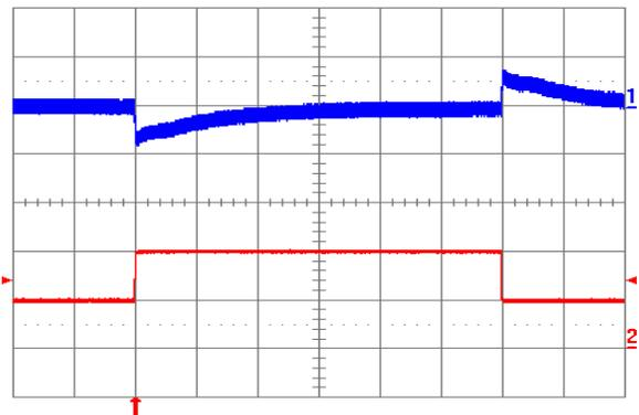
Fig. 6.0V.12: Output voltage response to load current step-change (2A - 4A - 2A) at  $V_{in} = 24\text{V}$ . Top trace: output voltage (100mV/div.). Bottom trace: load current (2A/div.). Current slew rate:  $5\ \text{A}/\mu\text{s}$ .  $C_o = 450\ \mu\text{F}$  tantalum +  $1\ \mu\text{F}$  ceramic. Time scale: 0.2 ms/div.
