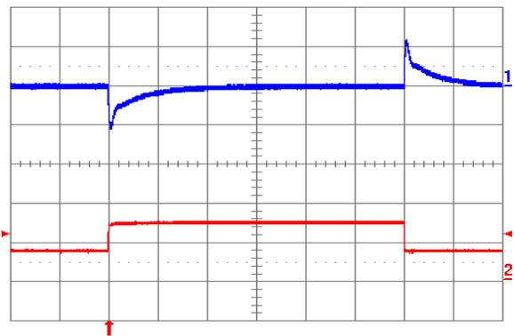
Fig. 1.2V.12: Output voltage response to load current step-change (3.75 A – 7.5 A – 3.75 A) at V<sub>in</sub> = 24V. Top trace: output voltage (100 mV/div.). Bottom trace: load current (5 A/div.). Current slew rate: 5 A/µs. C<sub>o</sub> = 450 µF tantalum + 1 µF ceramic. Time scale: 0.2 ms/div.
