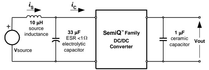
Fig. 2.0V.14: Test setup for measuring input reflected ripple currents,  $i_c$  and  $i_s$ .
