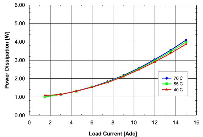
Fig. 1.0V.8: Power dissipation vs. load current and ambient temperature for SQ24T/S15010 converter mounted vertically with V<sub>in</sub> = 24V and air flowing from pin 3 to pin 1 at a rate of 200 LFM (1.0 m/s).
