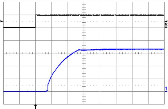
Fig. 3.3V.10: Turn-on transient at full rated load current (resistive) plus 10,000 µF at V<sub>in</sub> = 24V, triggered via ON/OFF pin. Top trace: ON/OFF signal (5 V/div.). Bottom trace: output voltage (1 V/div.). Time scale: 2 ms/div.
