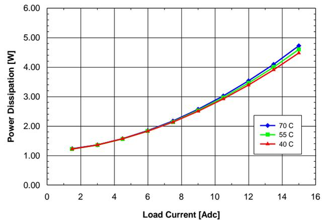
Fig. 1.5V.8: Power dissipation vs. load current and ambient temperature for SQ24T/S15015 converter mounted vertically with V<sub>in</sub> = 24V and air flowing from pin 3 to pin 1 at a rate of 200 LFM (1.0 m/s).
