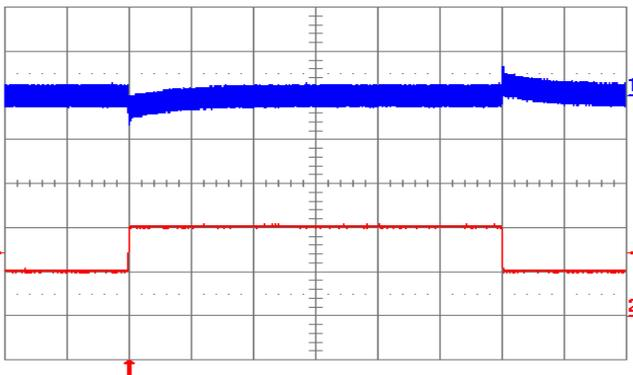
Fig. 12V.11: Output voltage response to load current step-change (1A – 2A – 1A) at  $V_{in} = 24\text{V}$ . Top trace: output voltage (200 mV/div.). Bottom trace: load current (1 A/div.). Current slew rate:  $0.1\text{ A}/\mu\text{s}$ .  $C_o = 1\ \mu\text{F}$  ceramic. Time scale: 0.5 ms/div.
