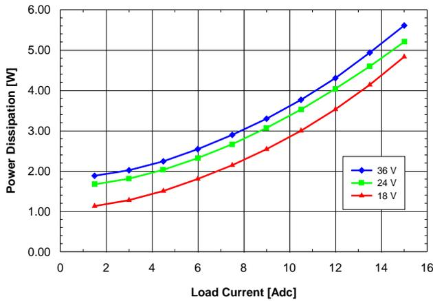
Fig. 2.0V.7: Power dissipation vs. load current and input voltage for SQ24T/S15020 converter mounted vertically with air flowing from pin 3 to pin 1 at a rate of 300 LFM (1.5 m/s) and T<sub>a</sub> = 25°C.
