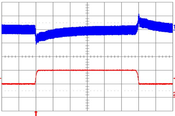
Fig. 6.0V.11: Output voltage response to load current step-change (2A - 4A - 2A) at  $V_{in} = 24\text{V}$ . Top trace: output voltage (100mV/div.). Bottom trace: load current (2A/div.). Current slew rate:  $0.1\ \text{A}/\mu\text{s}$ .  $C_o = 1\ \mu\text{F}$  ceramic. Time scale: 0.2 ms/div.
