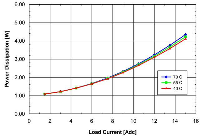
Fig. 1.2V.8: Power dissipation vs. load current and ambient temperature for SQ24T/S15012 converter mounted vertically with V<sub>in</sub> = 24V and air flowing from pin 3 to pin 1 at a rate of 200 LFM (1.0 m/s).
