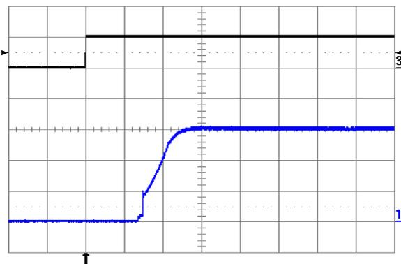
Fig. 1.5V.9: Turn-on transient at full rated load current (resistive) with no output capacitor at V<sub>in</sub> = 24V, triggered via ON/OFF pin. Top trace: ON/OFF signal (5 V/div.). Bottom trace: output voltage (0.5 V/div.). Time scale: 1 ms/div.
