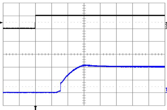
Fig. 1.0V.10: Turn-on transient at full rated load current (resistive) plus 10,000µF at V<sub>in</sub> = 24V, triggered via ON/OFF pin. Top trace: ON/OFF signal (5 V/div.). Bottom trace: output voltage (0.5 V/div.). Time scale: 1 ms/div.
