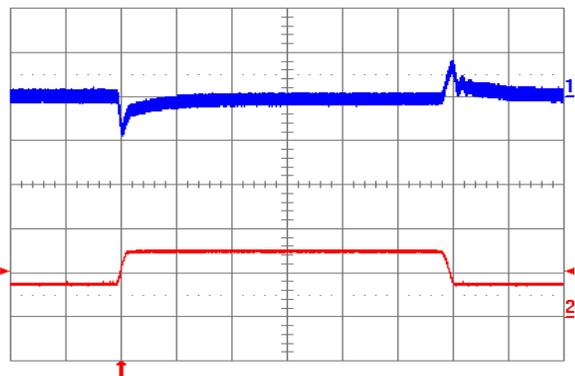
Fig. 1.8V.11: Output voltage response to load current step-change (3.75A – 7.5A – 3.75A) at  $V_{in} = 24\text{V}$ . Top trace: output voltage (100 mV/div.). Bottom trace: load current (5 A/div.). Current slew rate: 0.1 A/µs.  $C_o = 1\ \mu\text{F}$  ceramic. Time scale: 0.2 ms/div.
