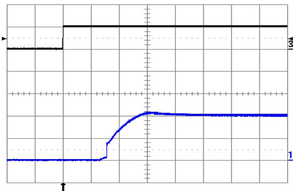
Fig. 1.0V.10: Turn-on transient at full rated load current (resistive) plus 10,000µF at V<sub>in</sub> = 24V, triggered via ON/OFF pin. Top trace: ON/OFF signal (5 V/div.). Bottom trace: output voltage (0.5 V/div.). Time scale: 1 ms/div.
