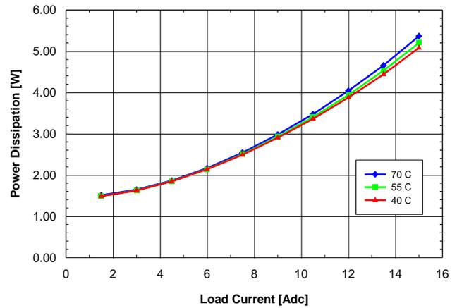
Fig. 2.0V.8: Power dissipation vs. load current and ambient temperature for SQ24T/S15020 converter mounted vertically with V<sub>in</sub> = 24V and air flowing from pin 3 to pin 1 at a rate of 200 LFM (1.0 m/s).
