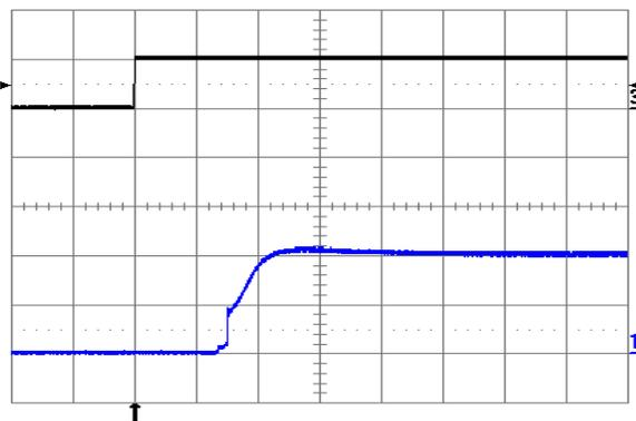
Fig. 1.0V.9: Turn-on transient at full rated load current (resistive) with no output capacitor at V<sub>in</sub> = 24V, triggered via ON/OFF pin. Top trace: ON/OFF signal (5 V/div.). Bottom trace: output voltage (0.5 V/div.). Time scale: 1 ms/div.
