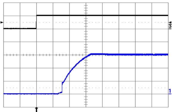
Fig. 1.5V.10: Turn-on transient at full rated load current (resistive) plus 10,000 µF at V<sub>in</sub> = 24V, triggered via ON/OFF pin. Top trace: ON/OFF signal (5 V/div.). Bottom trace: output voltage (0.5 V/div.). Time scale: 1 ms/div.
