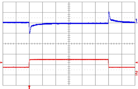
Fig. 1.8V.12: Output voltage response to load current step-change (3.75A – 7.5A – 3.75A) at  $V_{in} = 24\text{V}$ . Top trace: output voltage (100 mV/div.). Bottom trace: load current (5 A/div.). Current slew rate: 5 A/µs.  $C_o = 450\ \mu\text{F}$  tantalum + 1 µF ceramic. Time scale: 0.2 ms/div.
