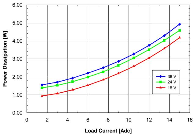
Fig. 1.5V.7: Power dissipation vs. load current and input voltage for SQ24T/S15015 converter mounted vertically with air flowing from pin 3 to pin 1 at a rate of 300 LFM (1.5 m/s) and T<sub>a</sub> = 25°C.
