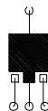
b. 95\text{ }^\circ\text{C/W} when mounted on a 0.066\text{ in}^2 pad of 2oz Cu.
