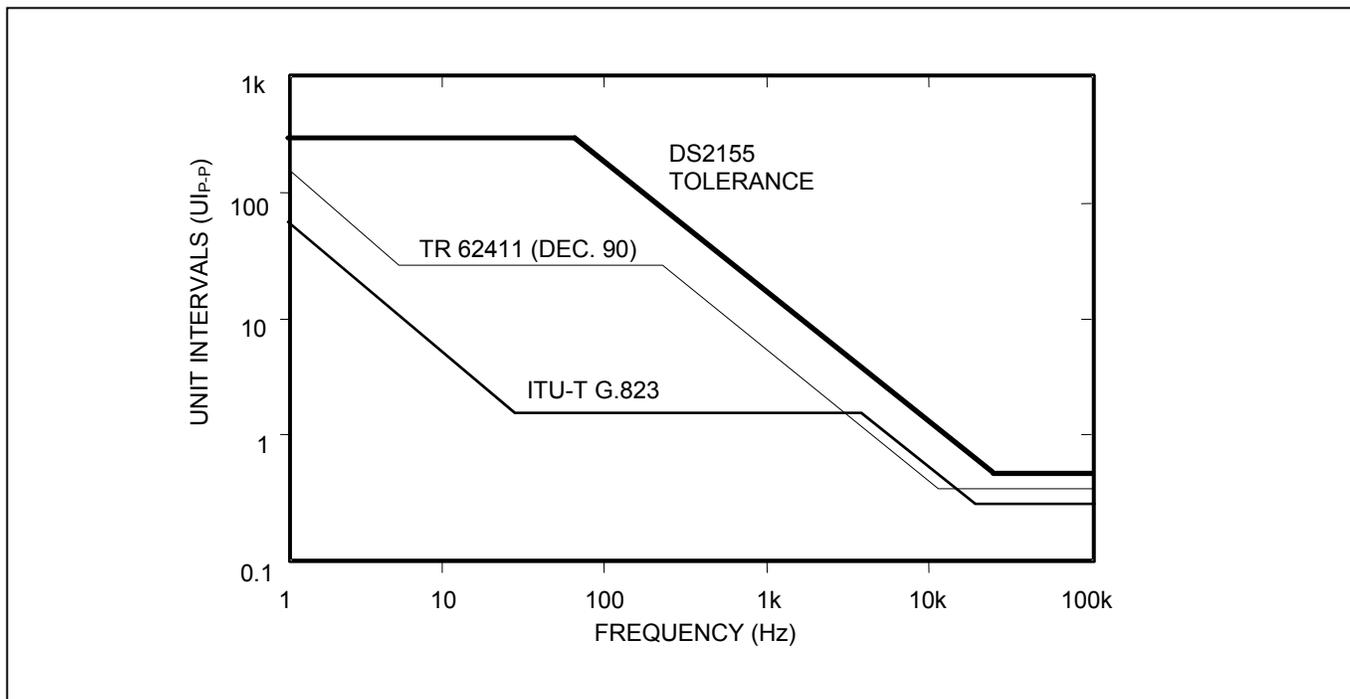
**Figure 24-8. Jitter Tolerance (E1 Mode)**
