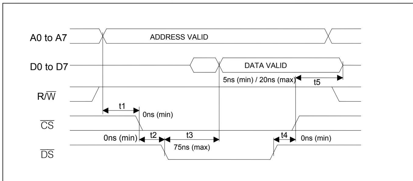
**Figure 37-7. Motorola Nonmultiplexed Bus Write Timing (BTS = 1/MUX = 0)**
