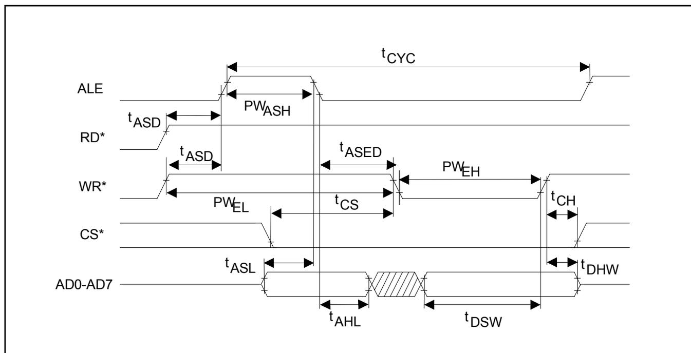
**Figure 37-3. Motorola Multiplexed Bus Timing (BTS = 1/MUX = 1)**
