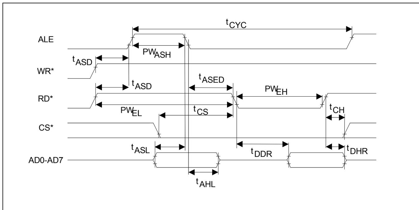
**Figure 37-2. Intel Multiplexed Bus Write Timing (BTS = 0/MUX = 1)**
