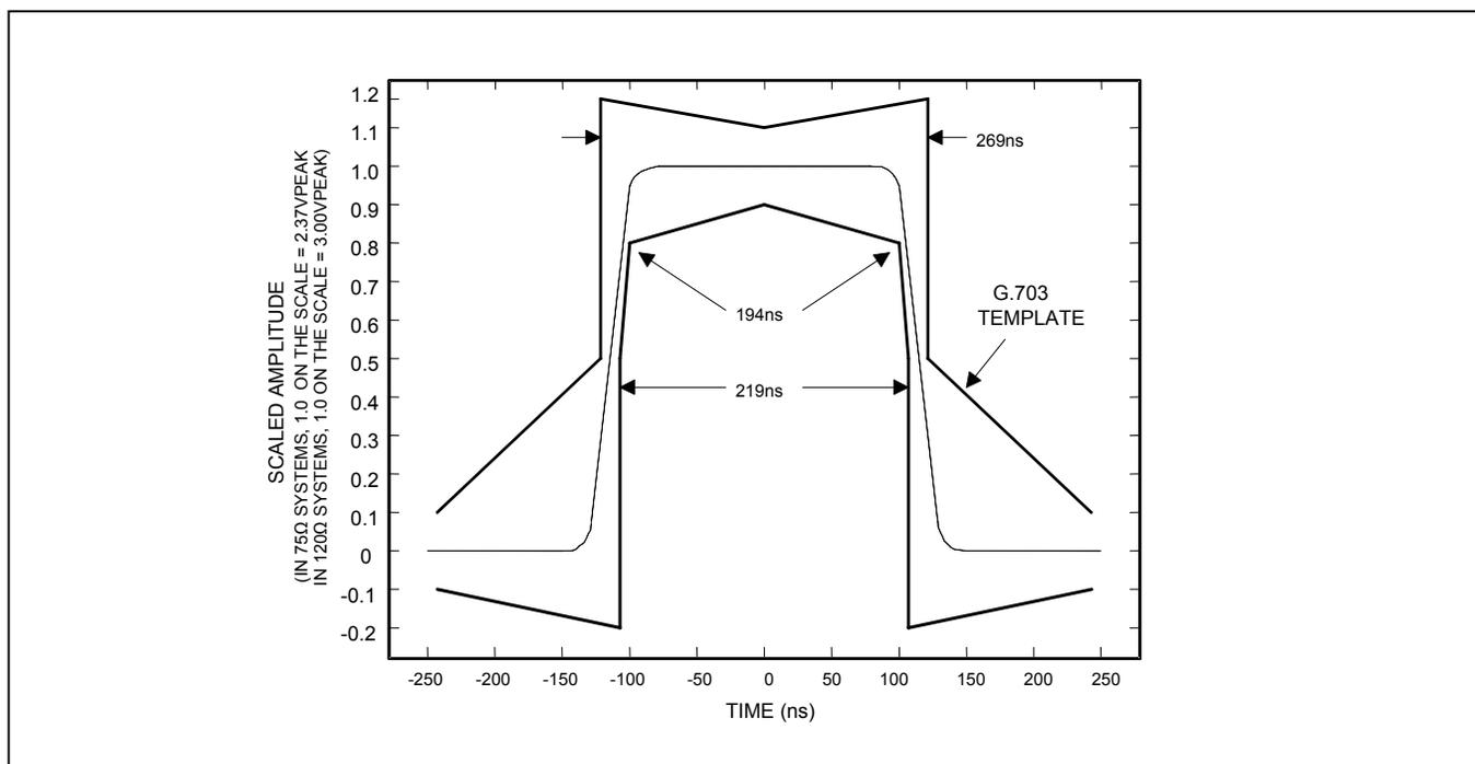
Figure 24-6. T1 Transmit Pulse Template
