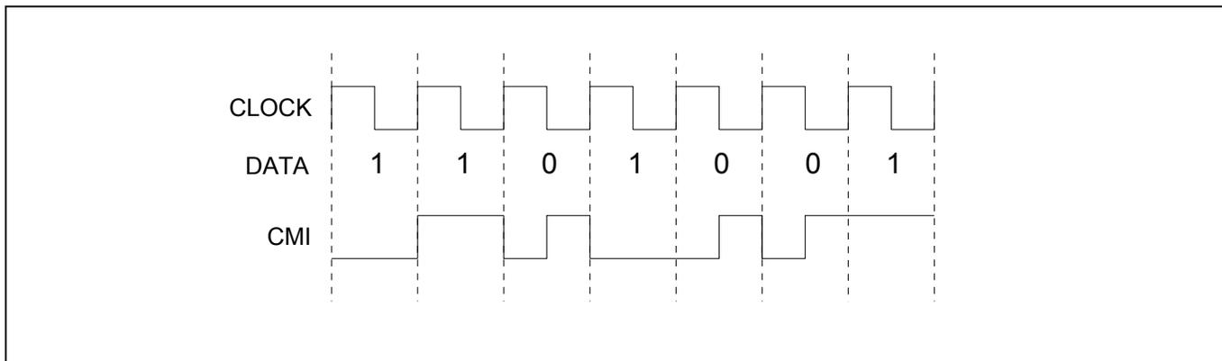
Transmit and receive CMI are enabled through LIC4.7. When this register bit is set, the TTIP pin outputs CMI-coded data at normal levels. This signal can be used to directly drive an optical interface. When CMI is enabled, the user can also use HDB3/B8ZS coding. When this register bit is set, the RTIP pin becomes a unipolar CMI input. The CMI signal is processed to extract and align the clock with data.
