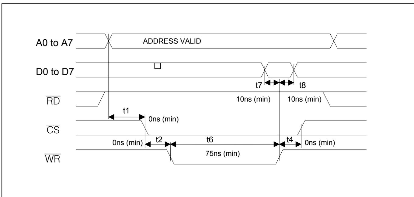
**Figure 37-6. Motorola Nonmultiplexed Bus Read Timing (BTS = 1/MUX = 0)**
