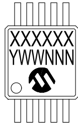
14-Lead SOIC (.150") (MCP624)
