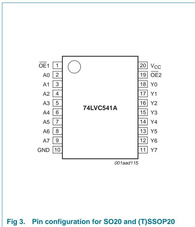
Fig 3. Pin configuration for SO20 and (T)SSOP20
