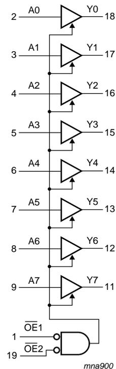
Fig 2. Functional diagram
