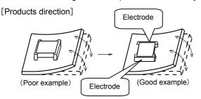
Products shall be located in the sideways direction (Length:a<b) to the mechanical stress.
