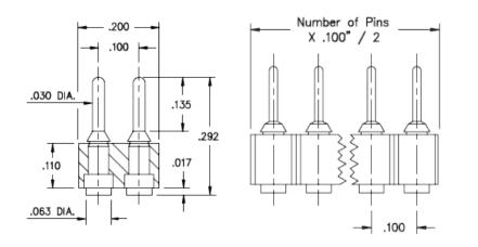
Description: Interconnect Header Surface Mount Pin Header .030" (0,76mm) Pin Head Double Row Surface Mount Plating Code: 10 Shell Plating: 10 μ" Gold over 100 μ" Nickel
