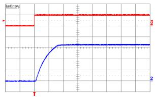
Figure 8: Output voltage response to load current step-change (10A–15A–10A) at Vin=48V. Top trace: output voltage (100 mV/div.). Bottom trace: load current (5Α/div.). Current slew rate: 0.1Α/μs. Co=1μF ceramic + 10μF tantalum. Time scale: 0.2mS/div.
