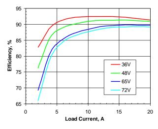
Figure 3: Efficiency vs. load current and ambient temperature for SSQE48T20033 converter mounted vertically with Vin=48V and air flowing from pin 1 to pin 3 at a rate of 200LFM (1.0m/s).
