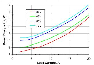
Figure 5: Power dissipation vs. load current and ambient temperature for SSQE48T20033 converter mounted vertically with Vin = 48 V and air flowing from pin 1 to pin 3at a rate of 200 LFM (1.0 m/s).
