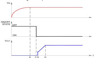
Scenario #3: Turn-off and Restart Using ON/OFF Pin
