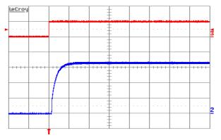
Figure 7: Turn-on transient at full rated load current (resistive) plus 20,000 μF at Vin = 48 V, triggered via ON/OFF pin. Top trace: ON/OFF signal (5 V/div.). Bottom trace: Output voltage (1 V/div.). Time scale: 5 mS/div.
