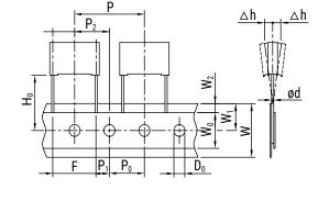
Figure 3 Lead Spacing 22.5 – 27.5 mm
