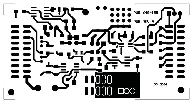
Figure 3. Layer 1 (Top Signal Plane)
