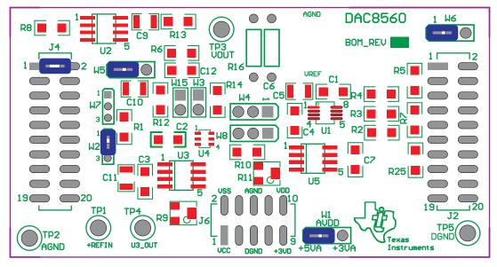
Figure 9. DAC8560EVM Default Jumper Configuration
