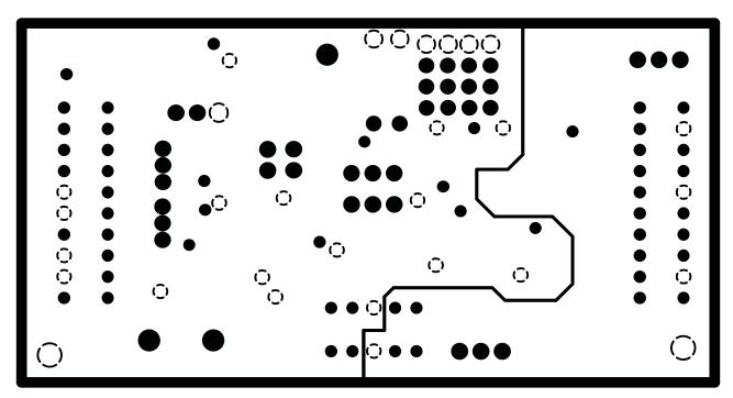
Figure 4. Layer 2 (Ground Plane)
