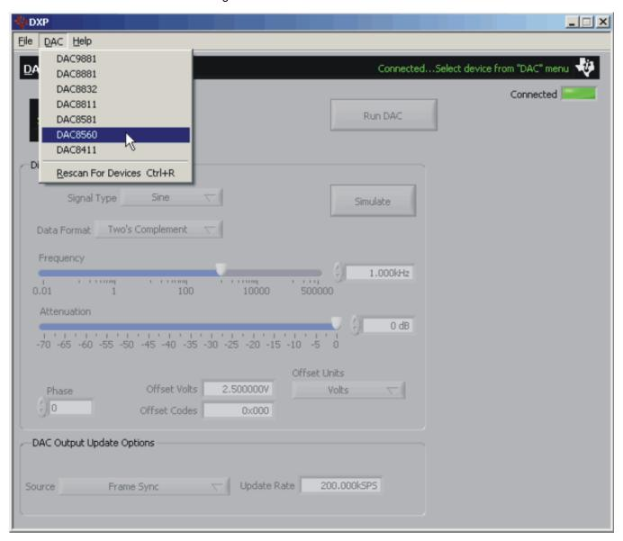
Figure 12. Loading a DAC8560EVM Configuration
