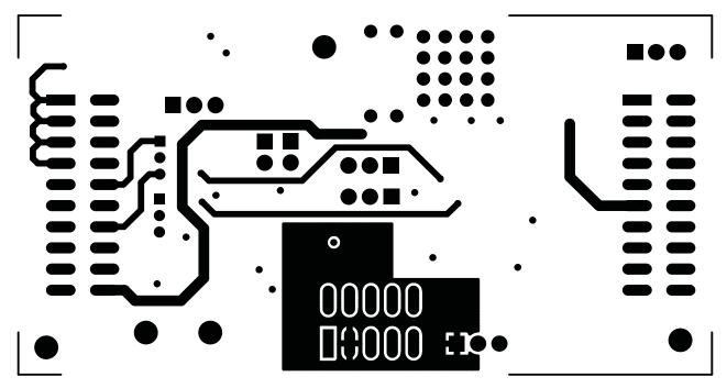
Figure 6. Layer 4 (Bottom Signal Plane)
