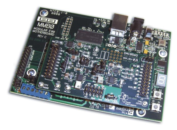
Figure 11. MMB0 with DAC8560EVM Installed
