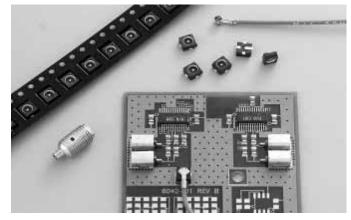
Microminiature surface mount cable assembly system designed to provide the performance of much larger industry-standard connectors.
