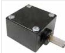
**LSXA - Standard:** 60° minimum overtravel, 15° maximum pretravel, 5° (single pole) and 7° (double pole) maximum differential travel.
