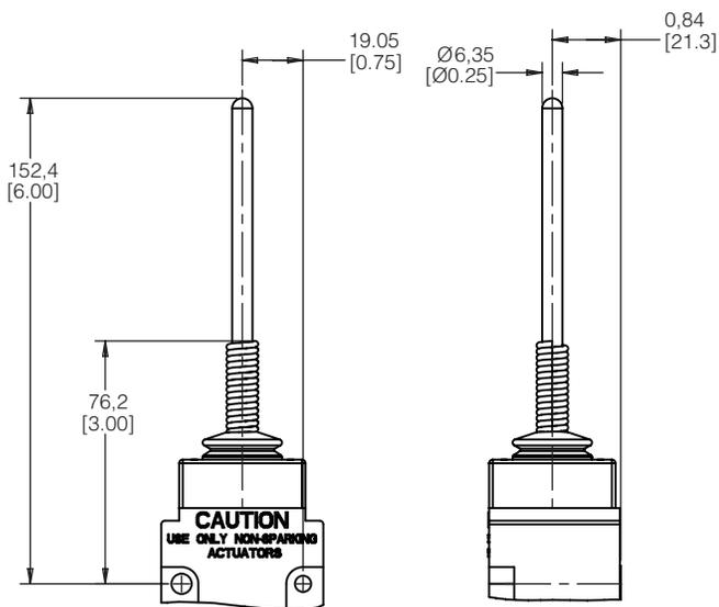
Figure 5. MICRO SWITCH™ LSX SERIES CAT WHISKER WOBBLE, HEAD CODE K • mm [in]
