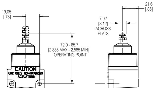
Figure 7. MICRO SWITCH™ LSX SERIES TOP PIN PLUNGER, HEAD CODE C • mm [in]
