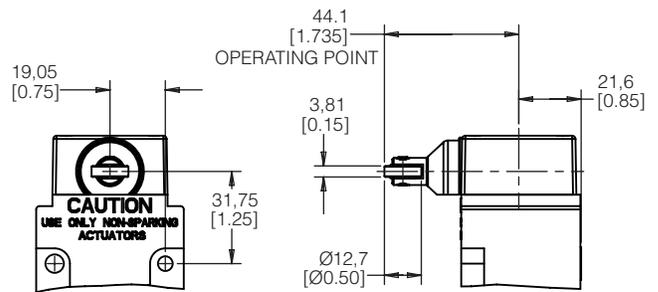
Figure 12. MICRO SWITCH™ LSX SERIES ADJUSTABLE SIDE PIN PLUNGER, HEAD CODE W • mm [in]
