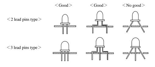
(2) Using spacer between LED's body and PCB is recommended.
