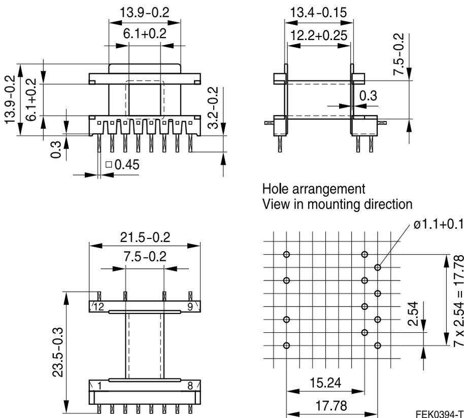
Figure 2, coil former (14 pins)
