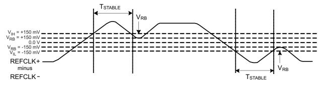
Figure 3. HCSL Ring Back Margin and Timing
