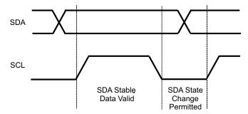
Figure 35. I<sup>2</sup>C Data/Address Bit Transmission
