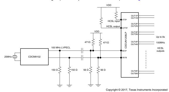
Figure 41. Clock Solution for PCle Express Applications
