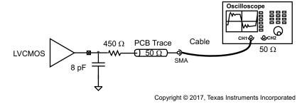
Figure 21. CDCUN1208LP LVCMOS Output - Measurement Configuration
