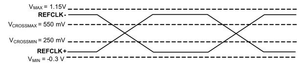
Figure 1. HCSL Crossing Point Voltage
