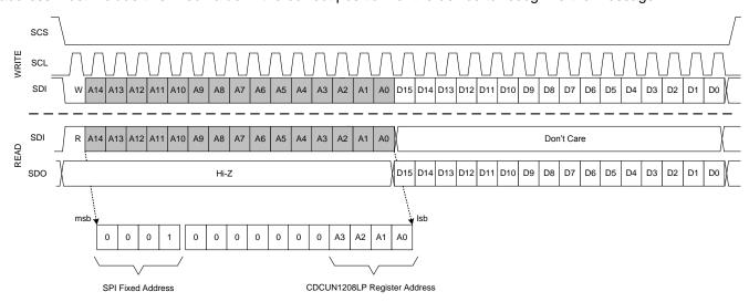
Figure 33. CDCUN1208LP Device Addressing - SPI Mode
