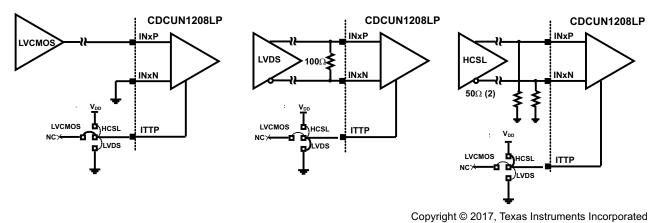
Figure 46. Common Interfaces to Device Inputs - DC Coupling
