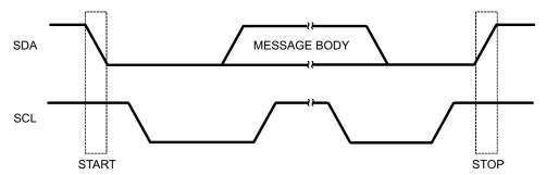
Figure 36. I<sup>2</sup>C Bus START and STOP Symbol Generation
