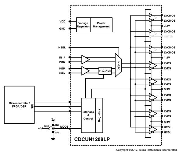
Figure 30. CDCUN1208LP Host Configuration – Typical Application
