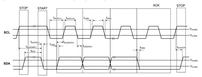
Figure 40. I<sup>2</sup>C Timing Diagram
