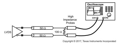
Figure 15. CDCUN1208LP LVDS Output - Test Setup
