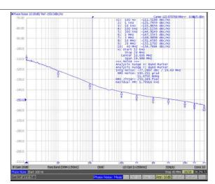
Figure 43. Output 2 (LVCMOS) Phase Noise With Clean 122.88-MHz Source
