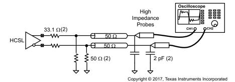
Figure 18. CDCUN1208LP HCSL Output - Measurement Configuration With Load
