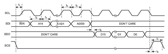
Figure 34. SPI Timing Diagram
