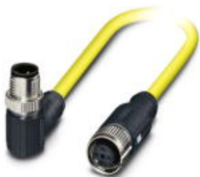
Sensor/actuator cable, 4-position, PVC, yellow, shielded, Plug angled M12 SPEEDCON, coding: A, on Socket straight M12 SPEEDCON, coding: A, cable length: 1.5 m
