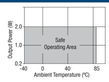
UL60950 recognition to a maximum ambient temperature of 85°C and/or case temperature limit of 155°C, measured on the face opposite the pins.
